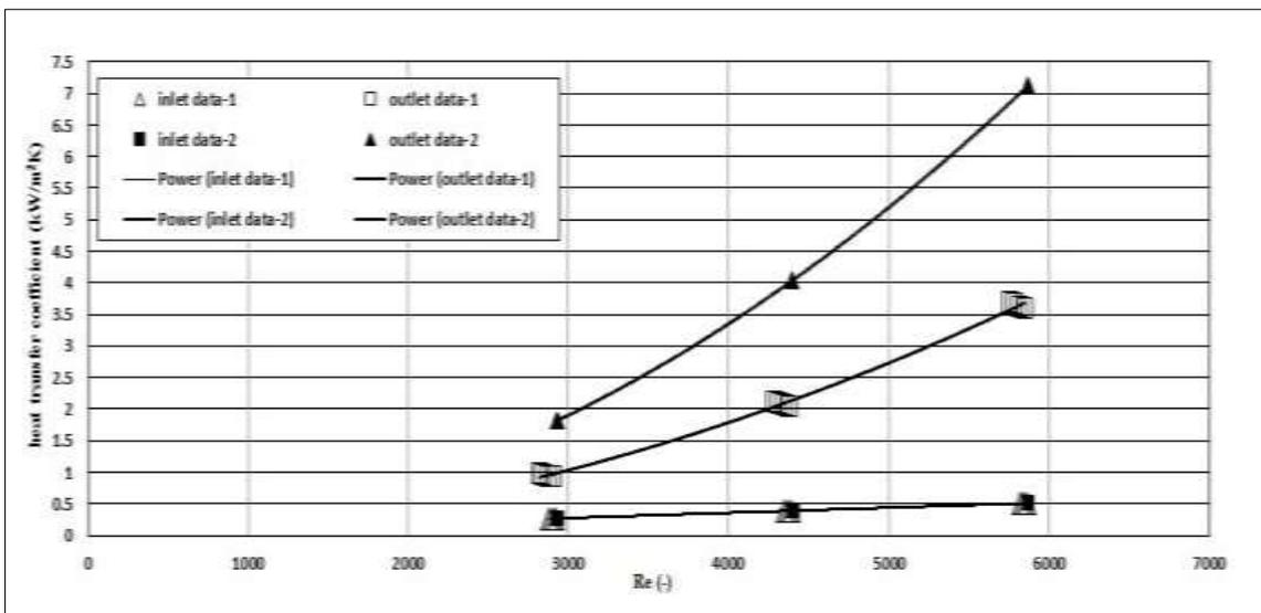
**Figure (4): Heat Transfer Coefficient versus Reynolds Number**
