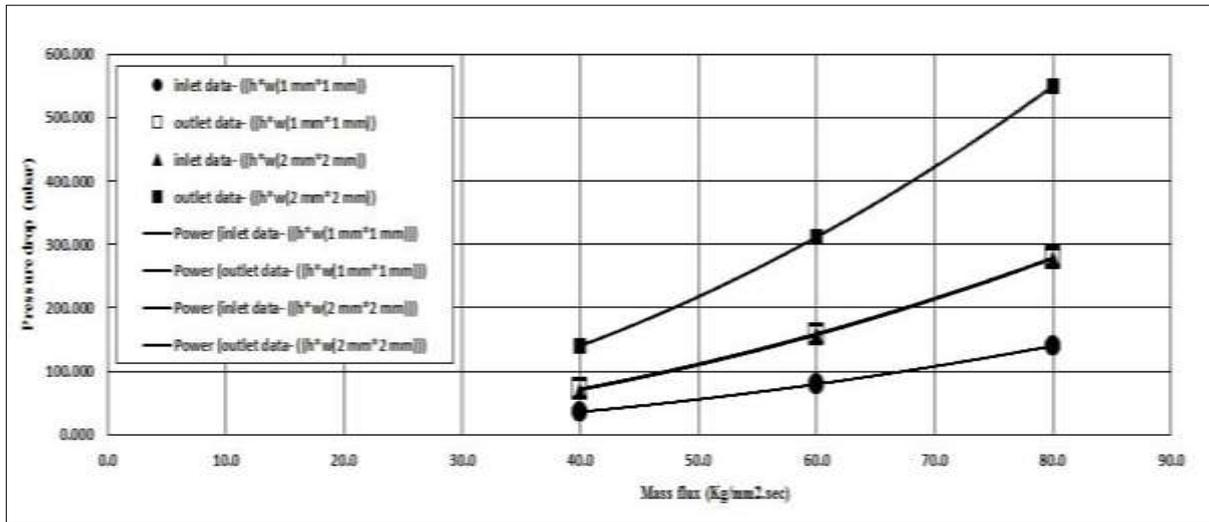
Figure (5): Relationship between Pressure Drop and Reynolds Number
