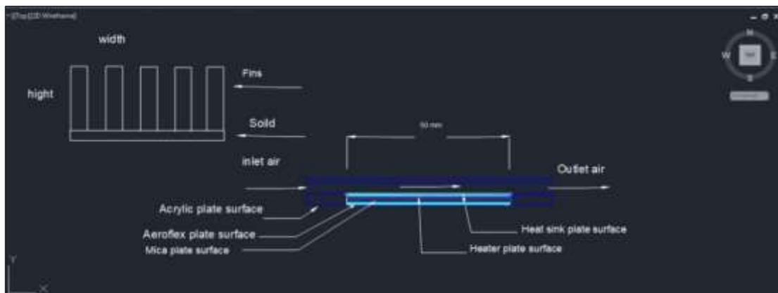
Figure (2): Experimental Segment and Test Component.[8]
