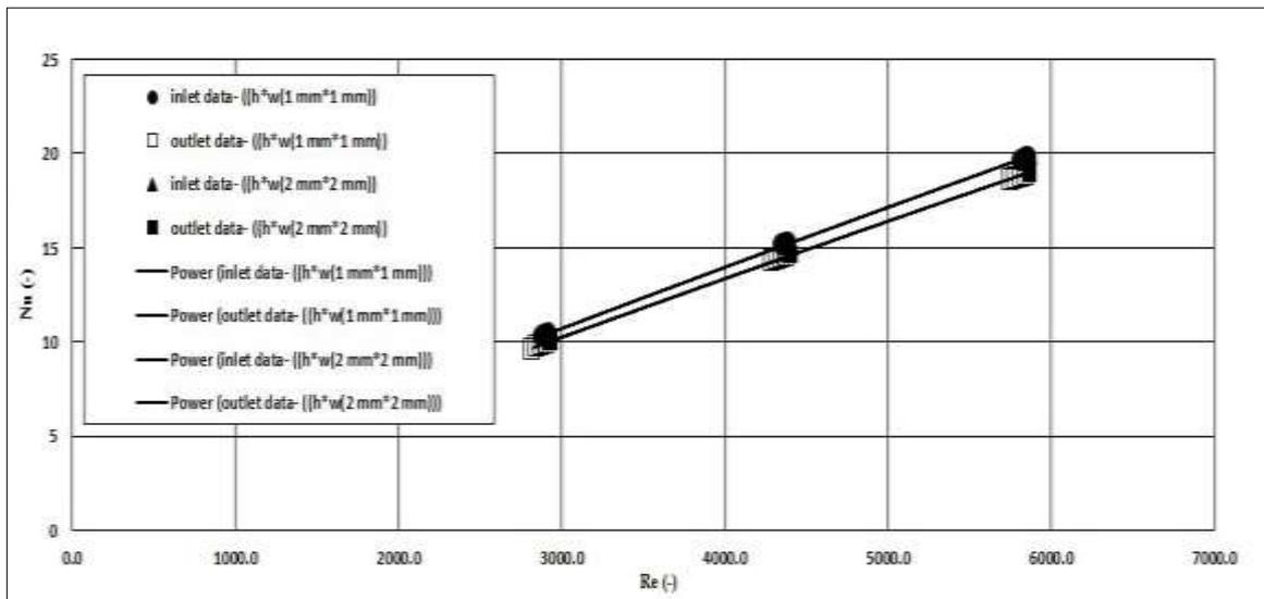
**Figure (7): Nusselt Number for Air versus Reynolds Number for Air**
