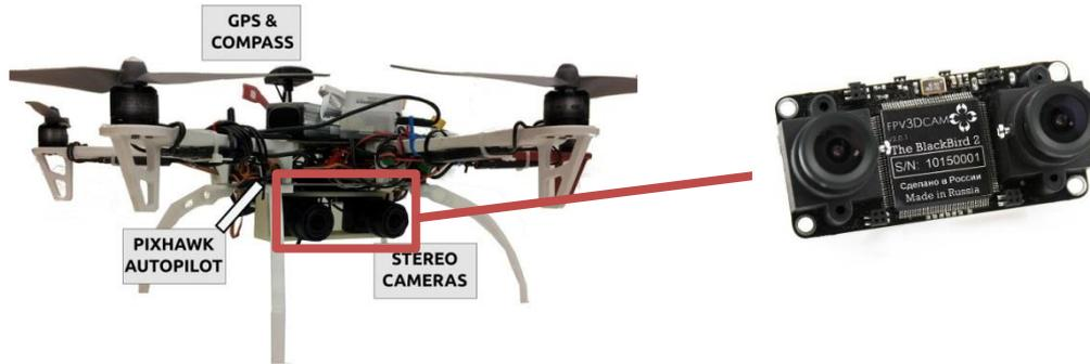
FIGURE 1 | DJI Drone (Left) being modified by the addition of the stereo camera (Right)
